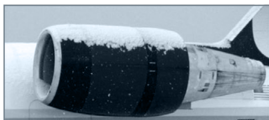
Aircraft parked without engine covers, allowing snow/ice accumulation inside the engine.
