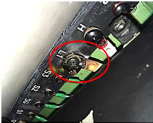
Sign of overheat on a windshield connector – Terminal lug stressed
