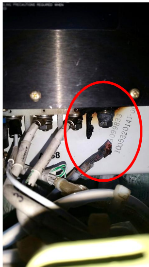
Electrical lug and WHTC stud damaged
