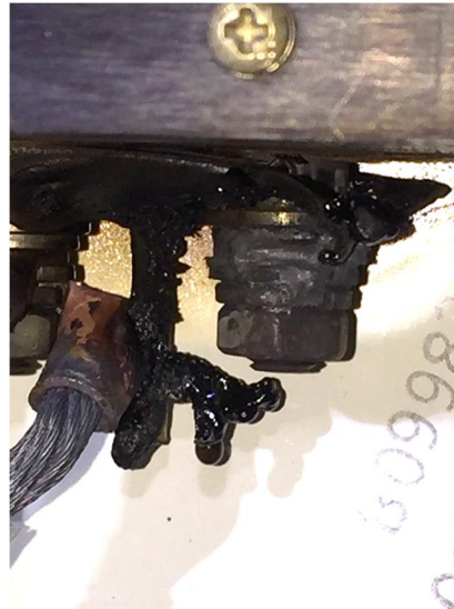
Electrical lug and WHTC stud damaged
