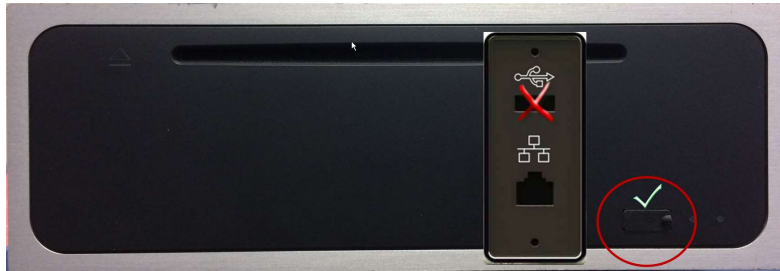
Figure 16: Correct USB port for Windows and terrain database updates
