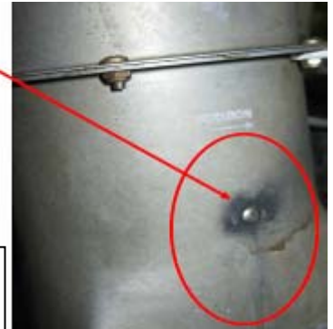
Notice hole is now elongated, allowing movement of the motor. This allows the fan blades (shown in next image) to make contact with the housing.
