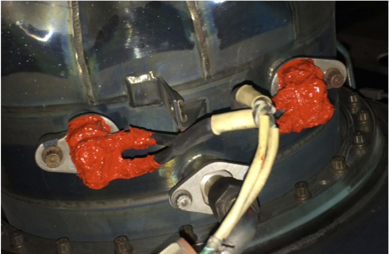
Figure 2. (Sheet 1 of 1) Proper RTV Sealant Application on the EGT Sensor and Electrical Wiring Harness
