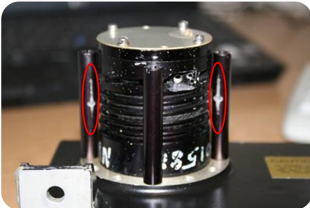
Figure 1 - Cable Keeper Wear
