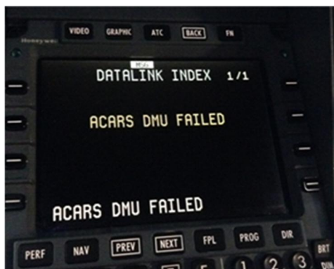
Figure 1 – 'ACARS DMU FAILED' messages displayed on FMS CDU
