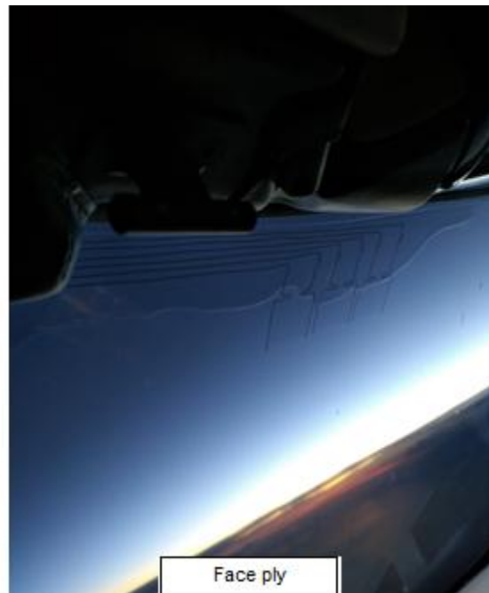
Figure 3: Main ply VS face ply delamination
