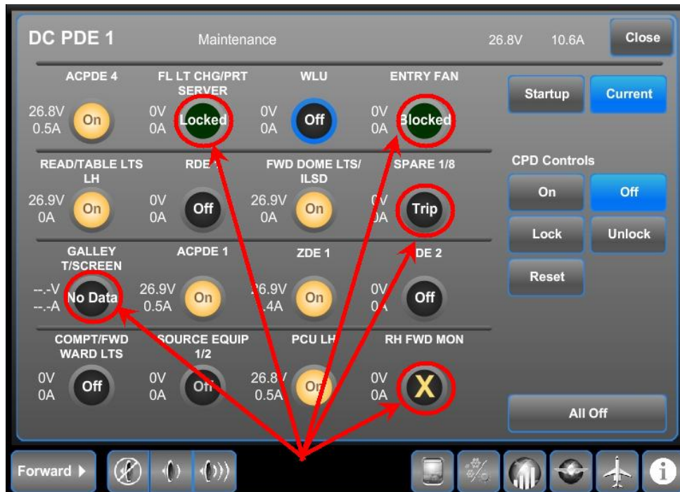
Figure 5, DC PDE Modes failures
