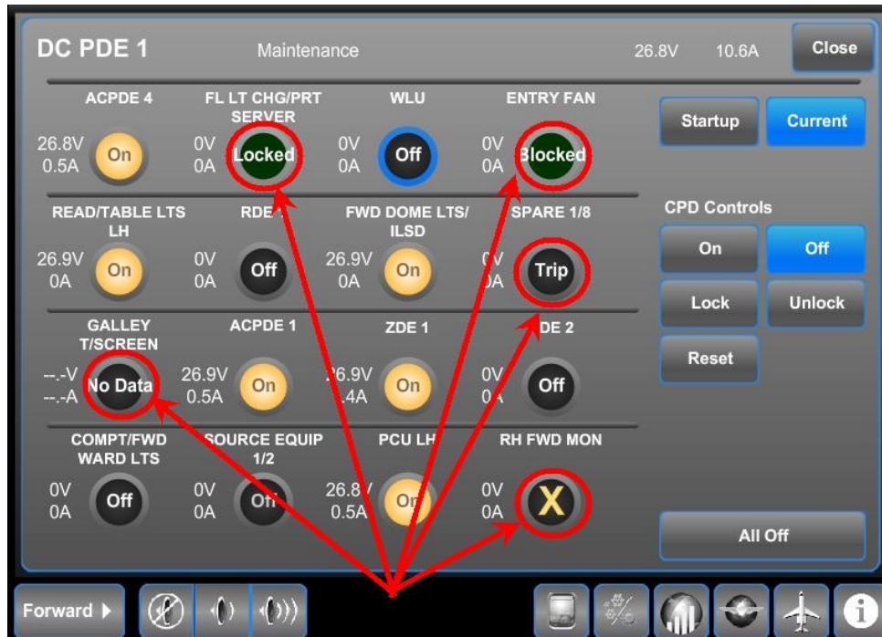
Figure 5, DC PDE Modes failures
